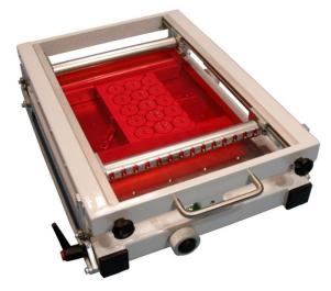
Clamp stencil through holes onto pins and screw up by front screws.
