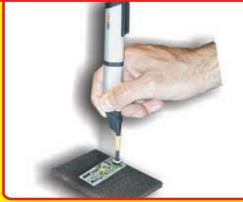
Micropic is designed to be held vertically and, with a pick nozzle in place, is used to pick and place components.
