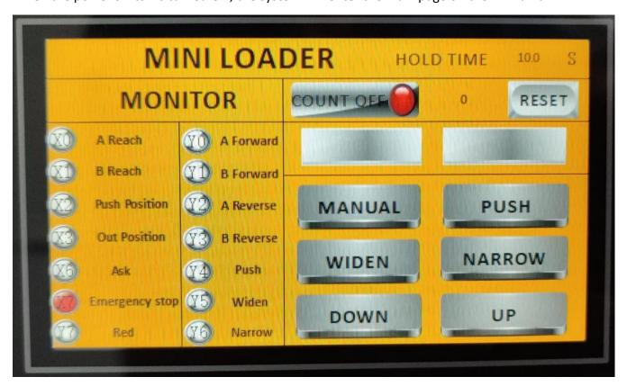
On the left side under Monitor the PLC information is displayed. Showing all the input signals X0...X7 and all output signals Y0...Y7
