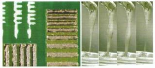
Before each addition the solder paste, the solder paste must be stirred uniformly before use, manual stirring speed is 2-3 seconds per revolution, in the same direction for 2 minutes to 5 minutes to make it into a fluid. The picture on the left is a typical printing abnormality caused by insufficient solder paste stirring. The picture on the right is a simple method for testing liquidity (Picking up solder paste with a stirring knife can naturally fall)
